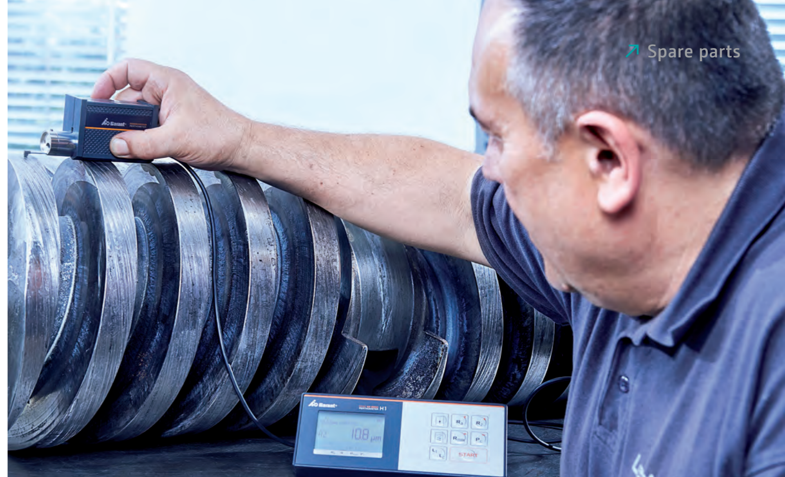
Our service employees carrying out a roughness measurement on a customer's spindle
