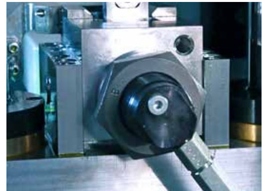
Hydraulic clamping system for the cutter bar
