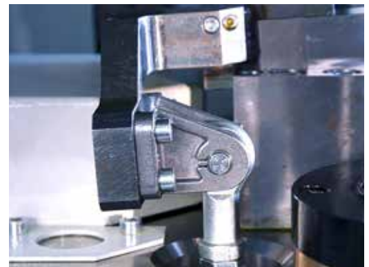
Hydraulic clamping system for the feed bar
