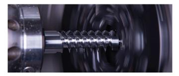
With whirling, helical profiles can be handled very efficiently. In this process, an eccentrically positioned whirling ring rotates around the slowly rotating work piece - in most cases without the use of a coolant. Because of the specific way of the cutting, the majority of the heat is discarded with the chip rather than heating up the workpiece.
