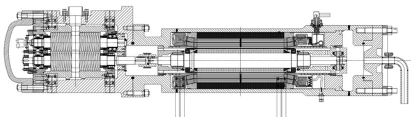
Figure 4. Subsea canned motor-pump.
