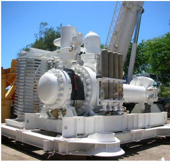
Figure 5. MPAM, retrievable motor pump module.
