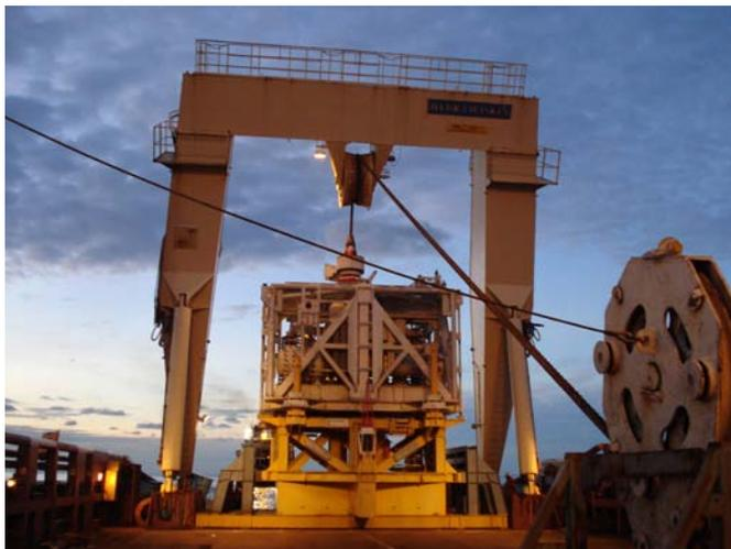
Figure 6. Subsea deployment using anchor handling vessel.
